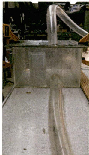
Figure 3C: One-way chamber control the direction of travel.
