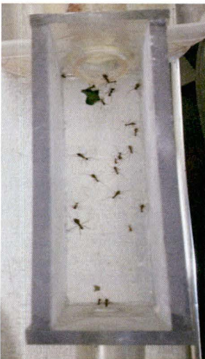
Figure 3A - Separation chamber allowing selection by category of ant.
