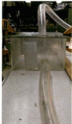
Figure 3C: One-way chamber control the direction of travel.
