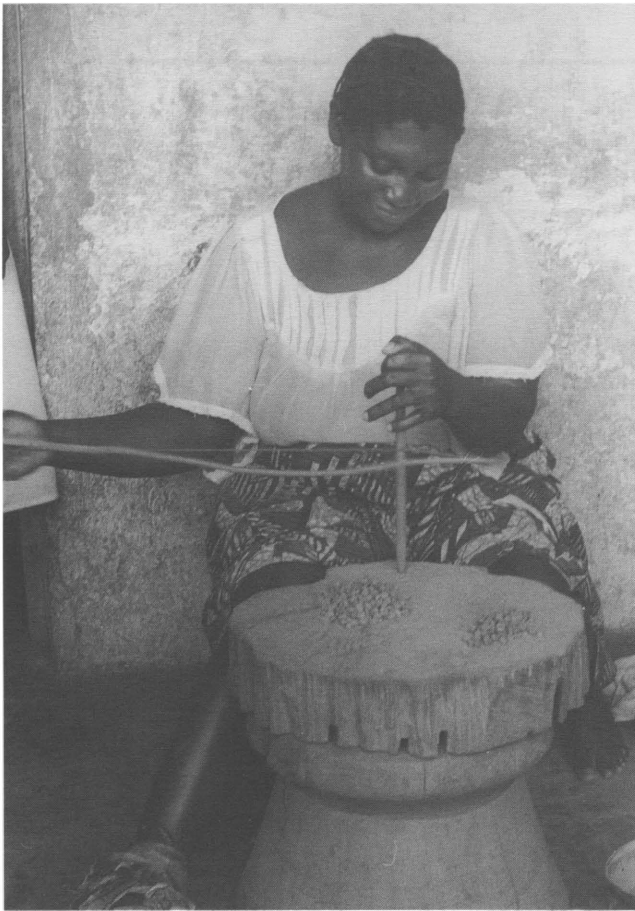
Figure 5. Drilling bead preforms with the bow-drill (photo: Bosman Murey).
