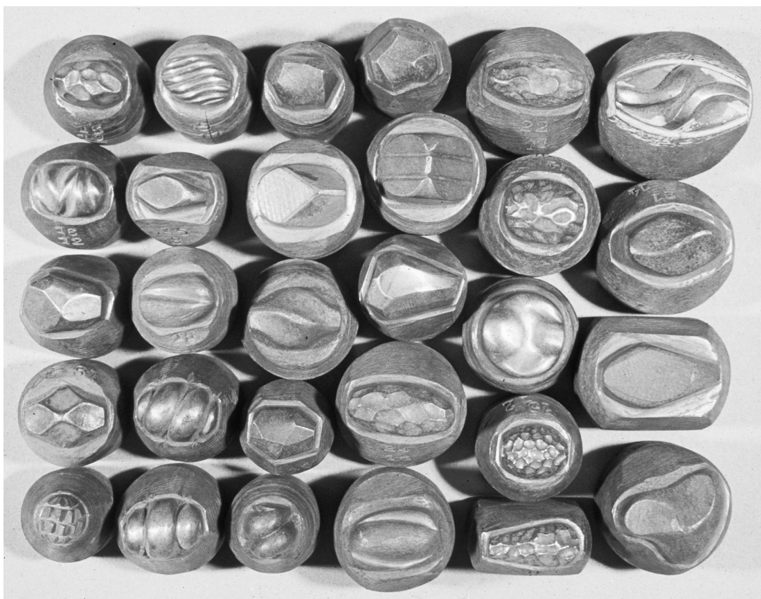
Figure 103. Molds for making “caps” for glass-pressing tongs (Adolf Glaser, mold-smith, Schwäbisch-Gmünd).
