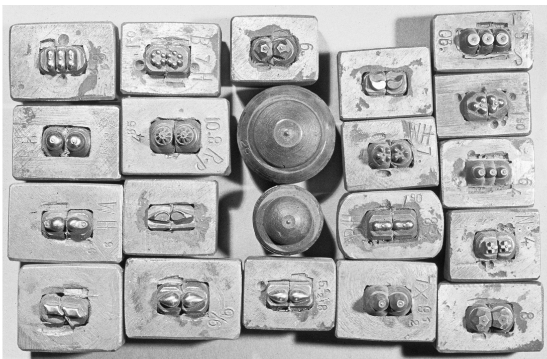
Figure 102. Molds for making “caps” for glass-pressing tongs (Adolf Glaser, mold-smith, Schwäbisch-Gmünd).
