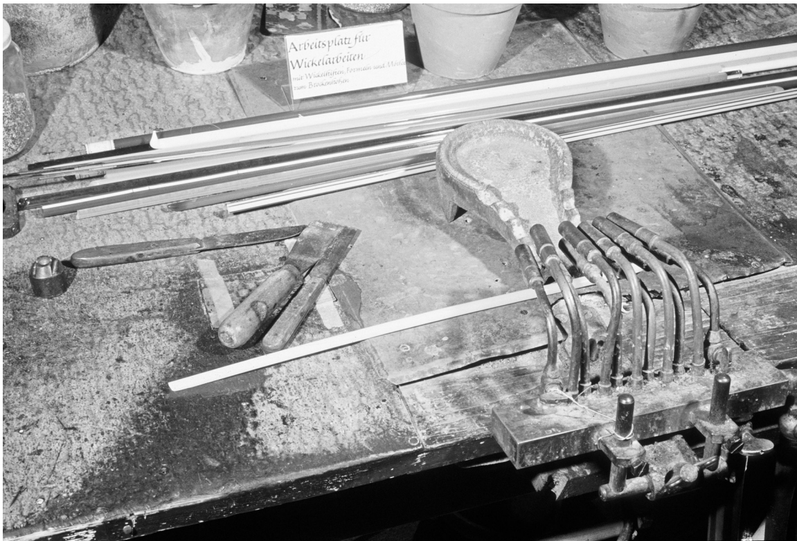
Figure 106. Work station for winding beads (using gas), Neugablonz, about 1950 (Neugablonz Industry and Jewelry Museum, Keufbeuren-Neugablonz).
