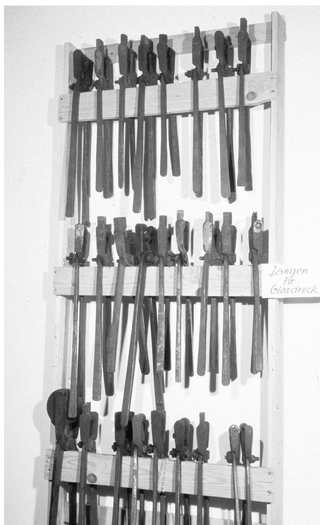
Figure 77. Press-molding tongs from various Neugablonz companies, 1948 (Neugablonz Industry and Jewelry Museum, Kaufbeuren-Neugablonz).
