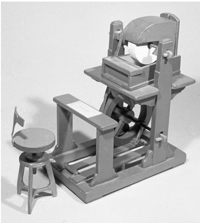
Figure 52. Model of treadle device (foot-driven grinder) (Gablonz Archive and Museum, Kaufbeuren-Neugablonz).
