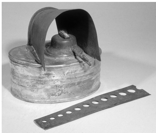
Figure 16. Lamp and measuring device for a blower of hollow glass beads; height (lamp): 11.3 cm; length (measuring device): 16.7 cm (Gablonz Archive and Museum, Kaufbeuren-Neugablonz).
