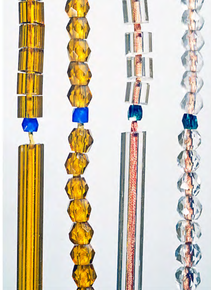
Plate 17B. Work stages for grinding (cutting) beads, topaz-colored glass (6-sided) and crystal glass (round); diameter (cane upper left): ca. 7.6 mm (TMV, probably TH 32842).
