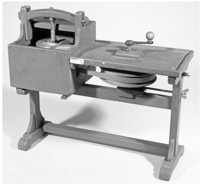
**Figure 63.** Model of an electrically driven grinding apparatus (Gablonz Archive and Museum, Kaufbeuren-Neugablonz).
