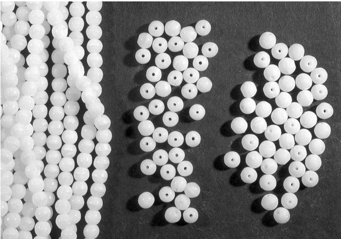
**Figure 83.** Stages in the manufacture of pressed beads (cf. Figure 82). From right to left: tumbled, polished, and strung beads; Heinz Kleinert, Neugablonz, 1977 (Gablonz Archive and Museum, Kaufbeuren-Neugablonz).
