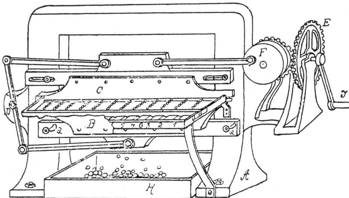
**Figure 122.** Device for segmenting beads (Parkert 1925:159, Figure 38).
