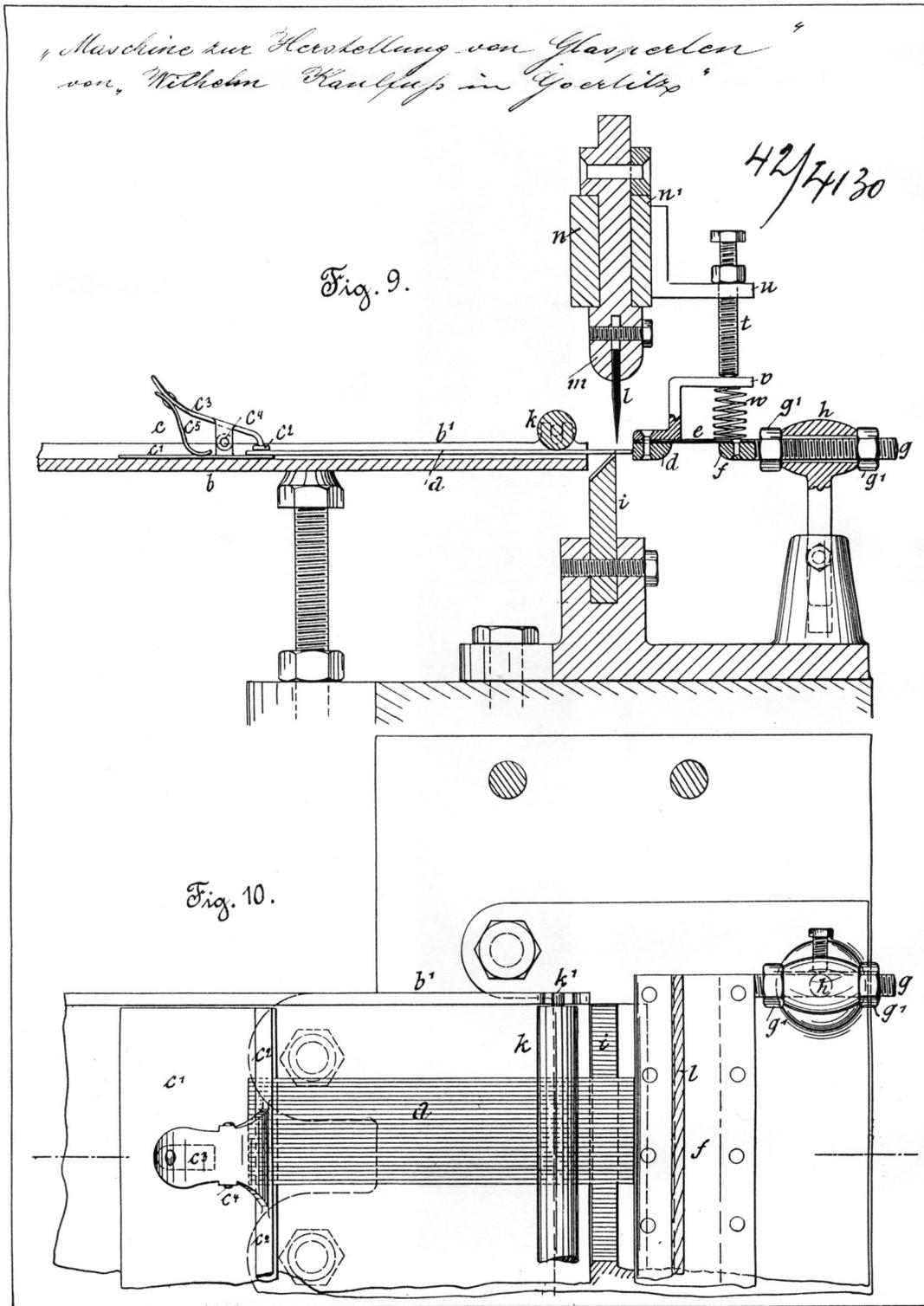
Figure 56b. Machine for making glass beads (Part 2).
