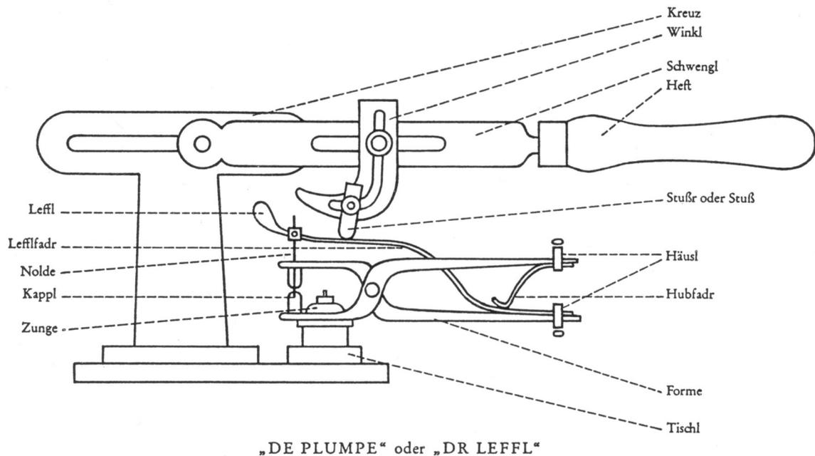
Figure 92. Molding tongs (“de Plumpe” or “dr Leffl”) (Kleinert 1972: Plate 1).
