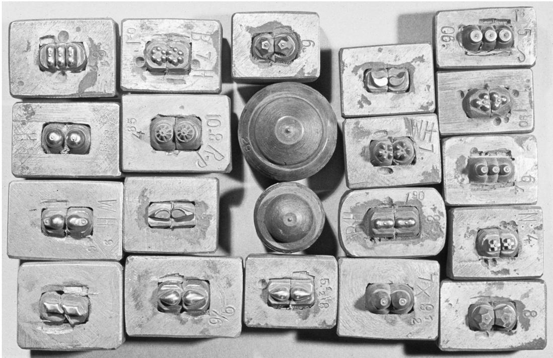
Figure 102. Molds for making “caps” for glass-pressing tongs (Adolf Glaser, mold-smith, Schwäbisch-Gmünd).
