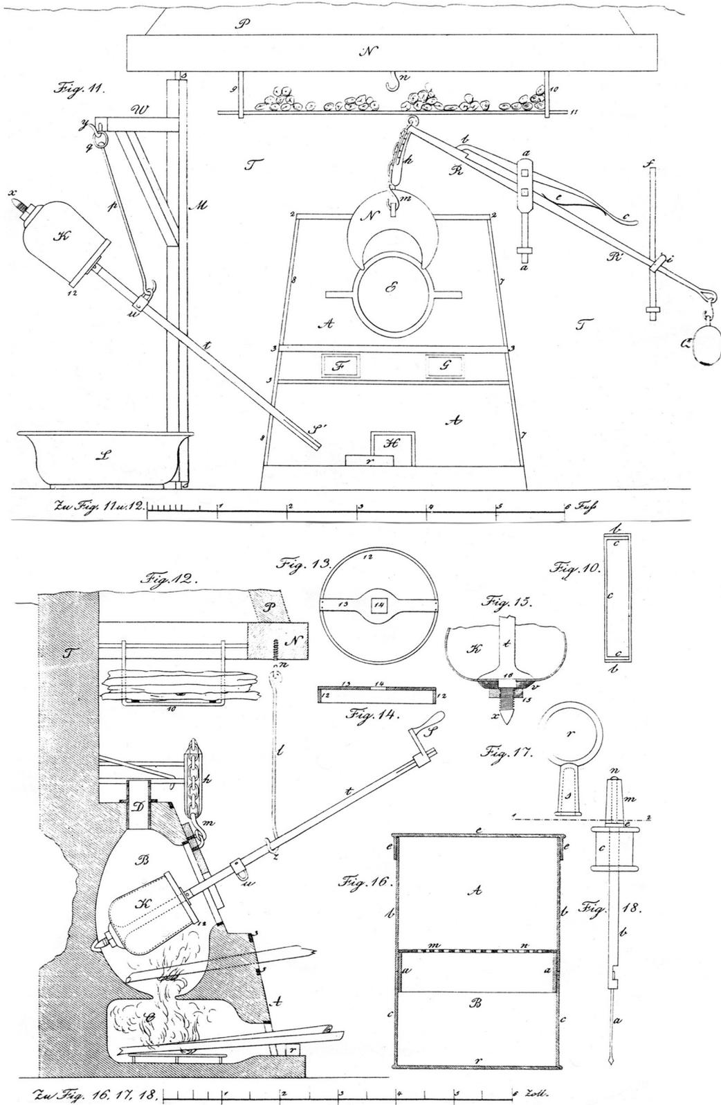
Figure 48. "New apparatus for rounding beads," probably after a privilege of Pusnich (Prechtl 1841, 11, and volume of illustrations, Plate 231).
