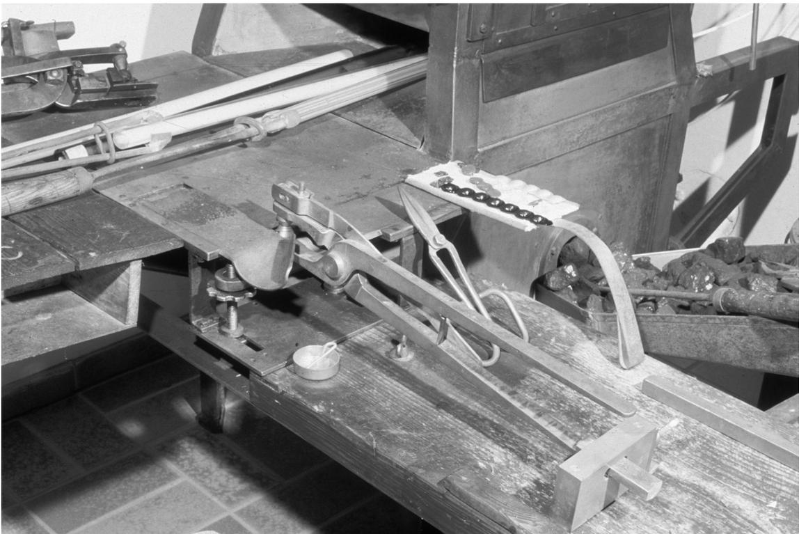
**Figure 85.** Work station at a press-molding factory (furnace, molding tongs).
