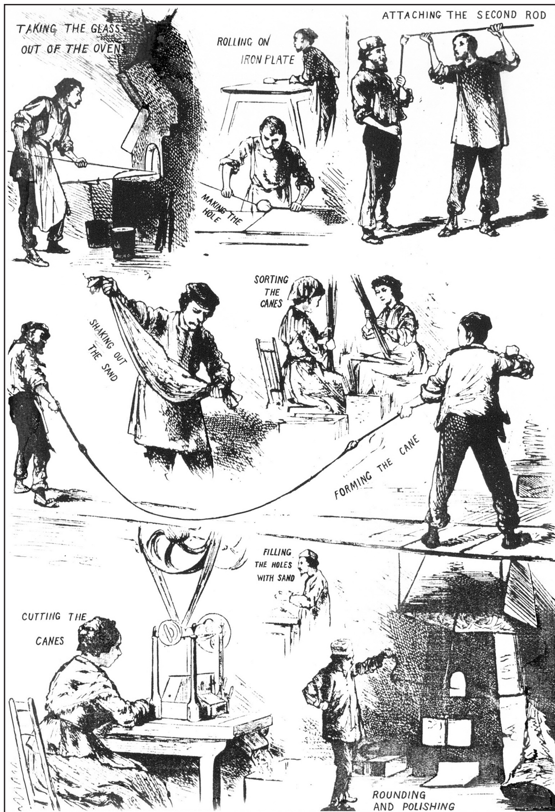
Figure 1. The various steps in drawn-bead production.
