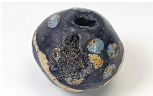
**Figure 6.** Imitation Type 6 bead exhibiting bubbling and a burned spot, having been overheated during the production process. The unusual black core is clearly visible (photo: Hans van der Storm).
