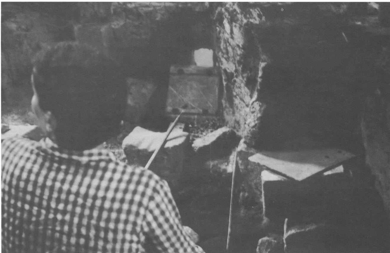
**Figure 2.** Glass beadmaking in Cairo, 1988. The setup is very similar to that used at Gorece, Turkey, and, other small beadmaking establishments, no doubt including Hebron. The beads are wound on the iron mandrel in the furnace, then removed to be shaped. When done they are knocked off into the small annealing chamber at the right. The blue beads in the center are rejects (photo by P. Francis, Jr.).
