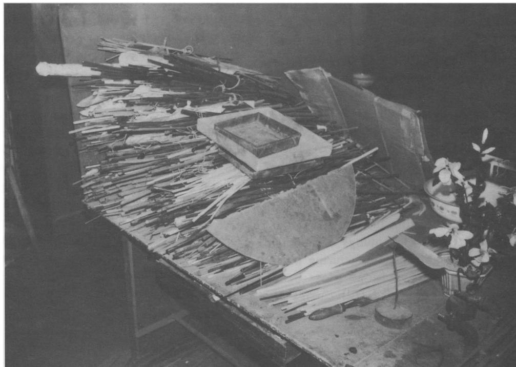
**Figure 2.** Glass rods used in the manufacture of glass objects at the Beijing Glass Ware Factory (photo by R. Sprague).
